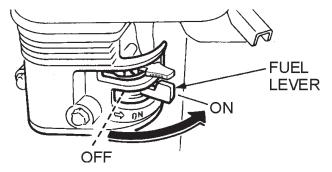
Figure 19. Fuel Valve Lever
